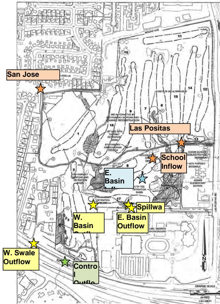
Figure 1. Project map with sampling stations. Orange represents stations for collecting inflow to the project, yellow represents sites downstream of treatment elements, green marks the control outflow site, and blue marks a site located between two treatment elements.
